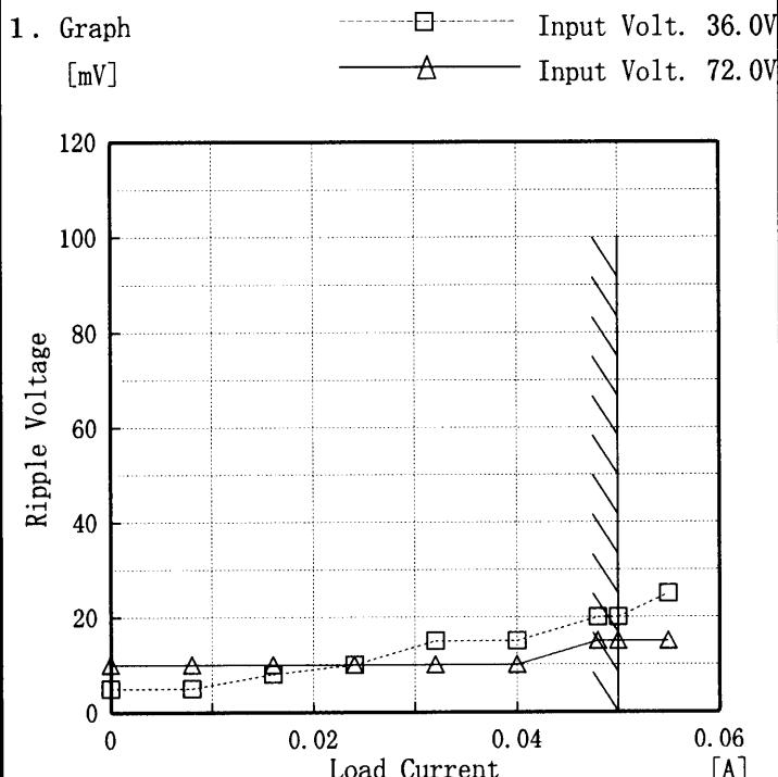
Ripple Voltage is shown as p-p in the figure below.
