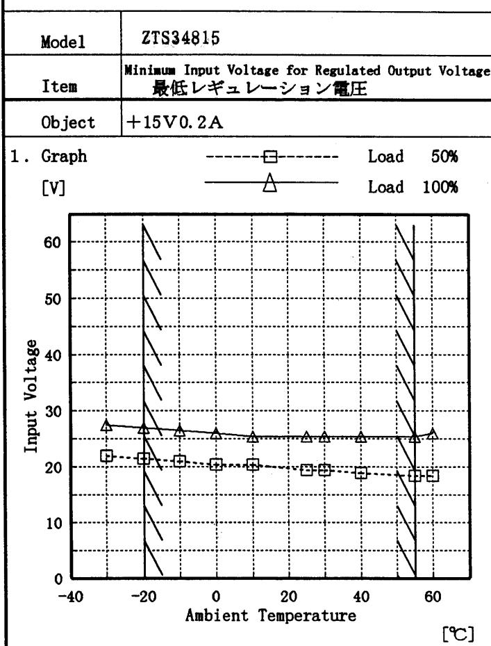
Note: Slanted line shows the range of the rated ambient temperature.
