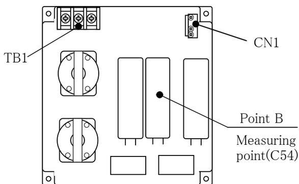
Fig.1 Measuring point(C54)
