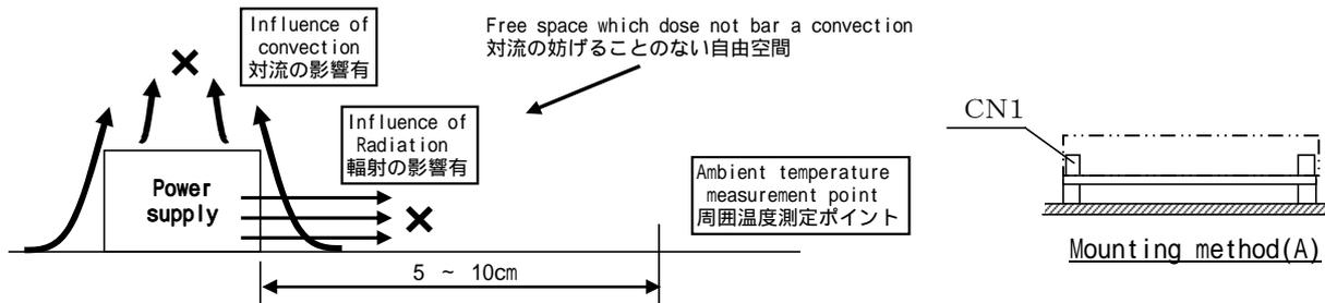
With the ambient temperature of graph, it measures in the environment of a figure.
