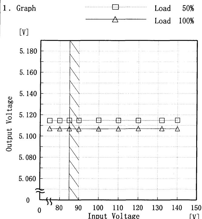
Note: Slanted line shows the range of the rated input voltage.
