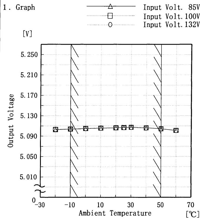
Note: Slanted line shows the range of the rated ambient temperature.
