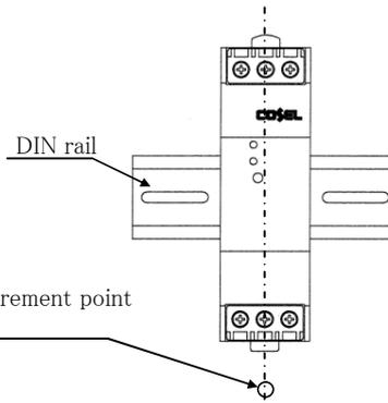
Ambient temperature measurement point
