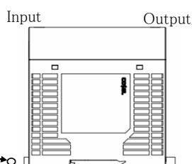
Ambient temperature measurement point
