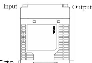
Ambient temperature measurement point
