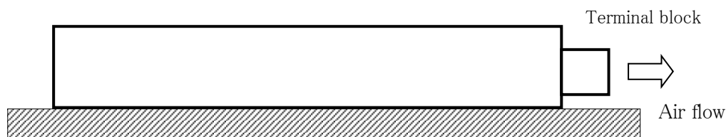
Fig.1.1 Mounting method (Normal position)
