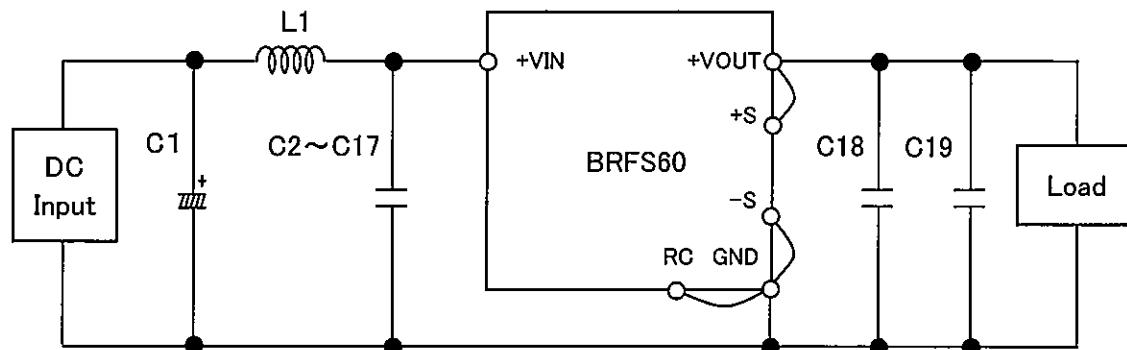
C1 : 25V       $470 \mu\text{F}$       Electrolytic capacitor
