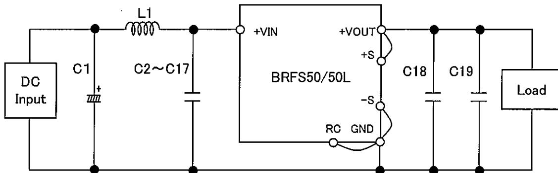
C1 : 25V       $220 \mu\text{F}$       Electrolytic capacitor
