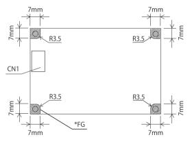
Recommend to electrically connect FG to metal chassis for reducing noise.
