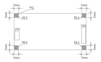
$\ensuremath{\bigstar}$  Recommend to electrically connect FG to metal chassis for reducing noise.
