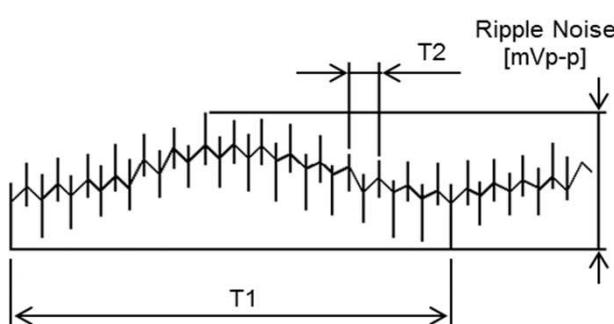
Fig. Complex Ripple Wave Form
