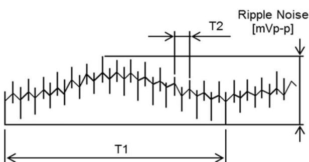
Fig. Complex Ripple Wave Form
