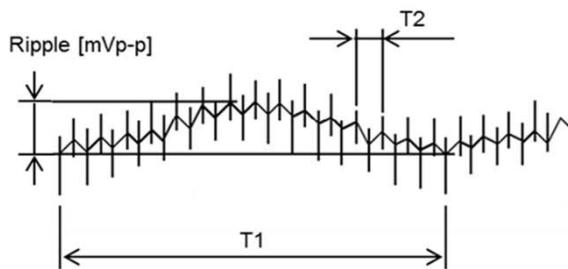
Fig. Complex Ripple Wave Form
