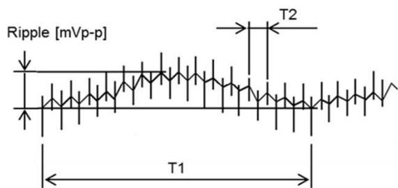
Fig. Complex Ripple Wave Form
