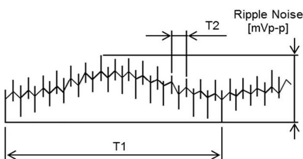
Fig. Complex Ripple Wave Form
