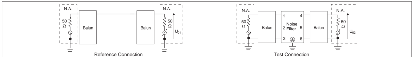
Fig.3.3 Differential mode attenuation measurement diagram
