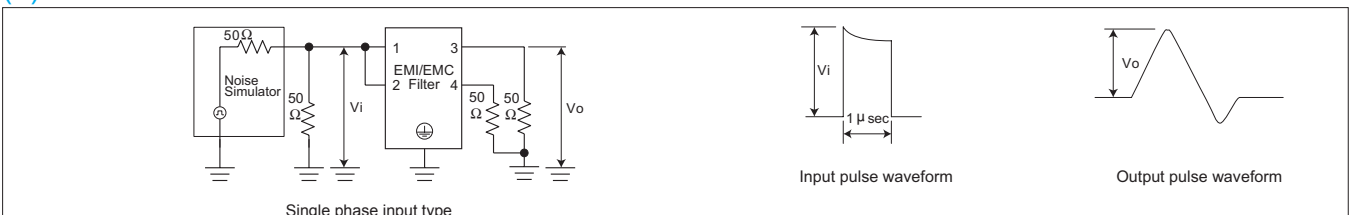
Fig.3.7 Pulse attenuation measurement diagram
