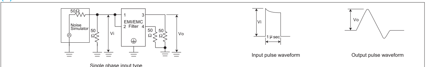
Fig.3.7 Pulse attenuation measurement diagram
