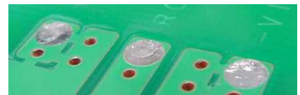
Fig. 5.1.1.2 The pad after solder removal
