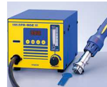
Fig. 3.4.2.5 Hot Air HAKKO FR-802 (model name)
