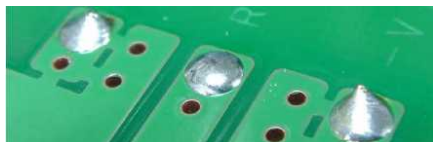
Fig. 5.1.1.1 The pad after power supply removal
