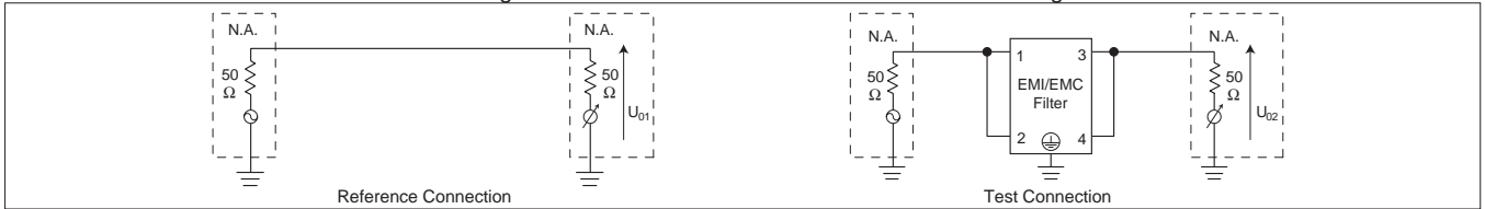
Fig.3.2 Common mode attenuation measurement diagram
