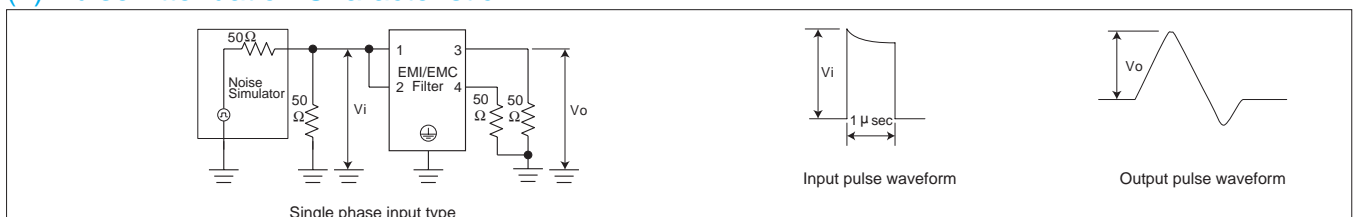
Fig.3.7 Pulse attenuation measurement diagram
