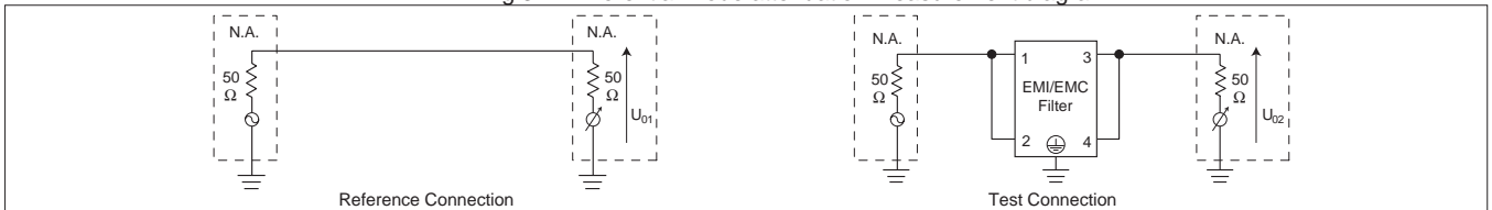
Fig.3.2 Common mode attenuation measurement diagram
