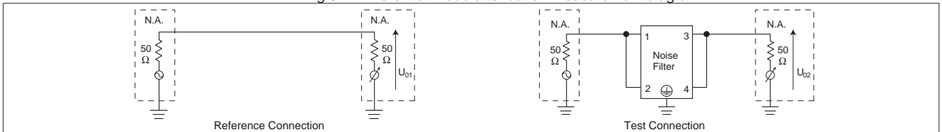
Fig.3.2 Common mode attenuation measurement diagram
