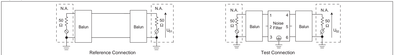
Fig.3.3 Differential mode attenuation measurement diagram
