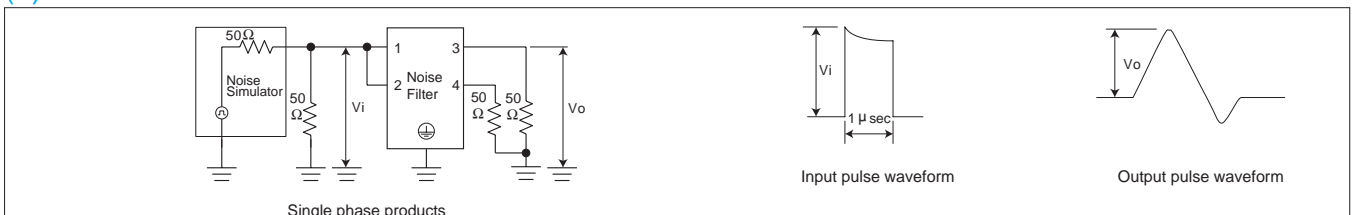
Fig.3.7 Pulse attenuation measurement diagram
