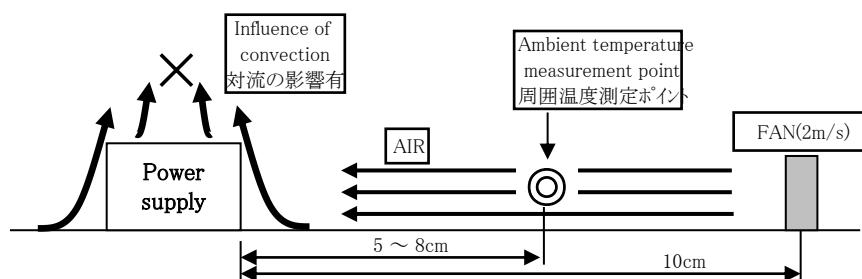
With the ambient temperature of graph, it measures in the environment of a figure.
